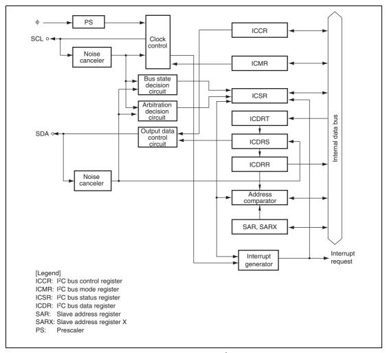
Figure 15.1 Block Diagram of I<sup>2</sup>C Bus Interface
