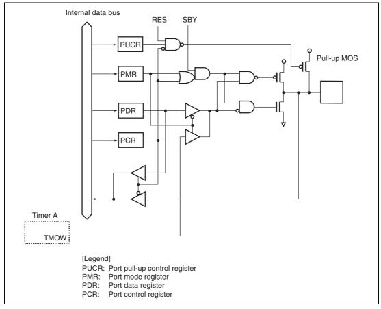
Figure B.4 Port 1 Block Diagram (P10)
