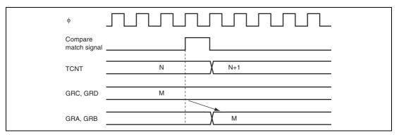
**Figure 12.19 Buffer Operation Timing (Compare Match)**
