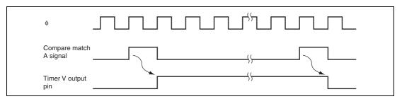
Figure 11.6 TMOV Output Timing
