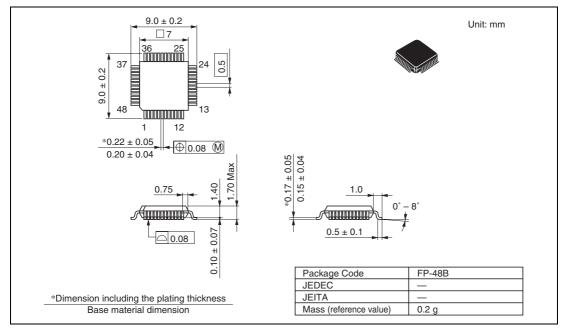
Figure D.4 FP-48B Package Dimensions
