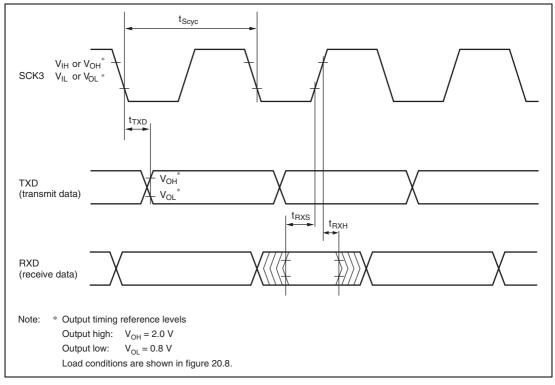
Figure 20.6 SCI3 Input/Output Timing in Clocked Synchronous Mode
