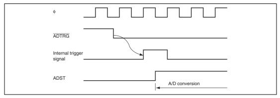
Figure 16.3 External Trigger Input Timing
