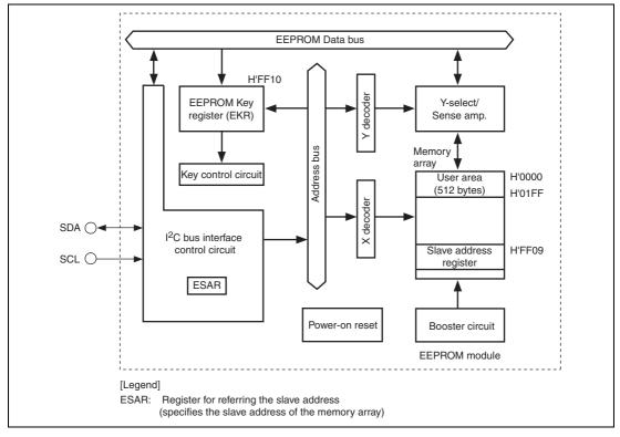
Figure 17.1 Block Diagram of EEPROM
