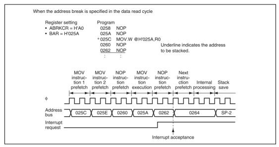
Figure 4.2 Address Break Interrupt Operation Example (2)
