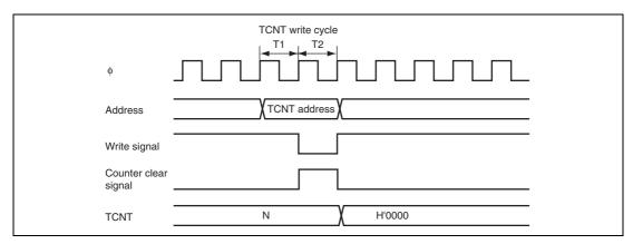
Figure 12.24 Contention between TCNT Write and Clear
