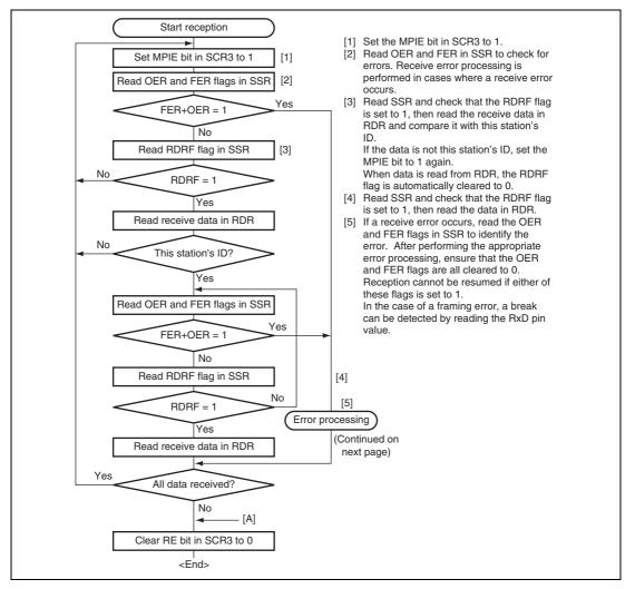
Figure 14.17 Sample Multiprocessor Serial Reception Flowchart (1)
