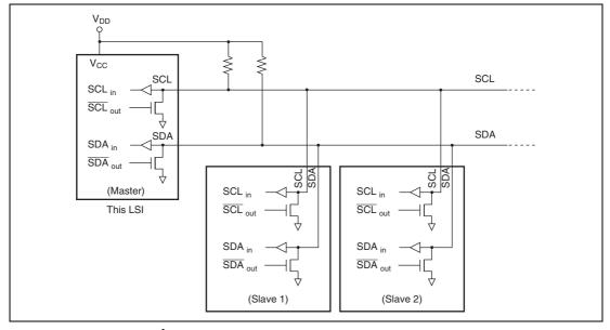
Figure 15.2 I<sup>2</sup>C Bus Interface Connections (Example: This LSI as Master)
