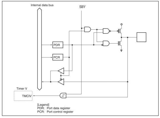
Figure B.12 Port 7 Block Diagram (P75)
