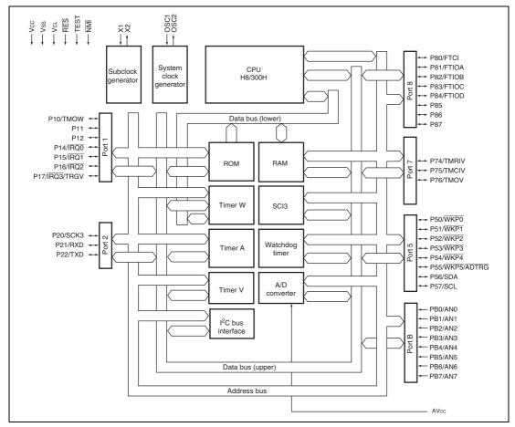
Figure 1.1 Internal Block Diagram of H8/3664 of F-ZTAT<sup>™</sup> and Mask-ROM Versions
