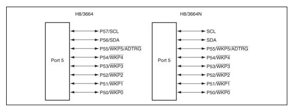
Figure 9.3 Port 5 Pin Configuration
