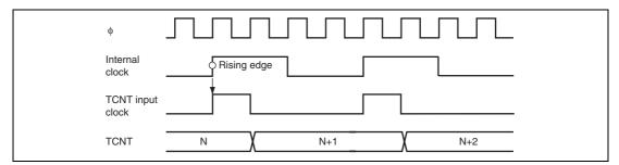
Figure 12.14 Count Timing for Internal Clock Source
