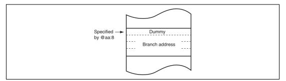
Figure 2.8 Branch Address Specification in Memory Indirect Mode
