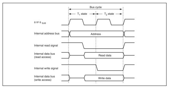
Figure 2.9 On-Chip Memory Access Cycle
