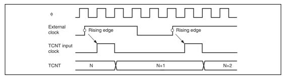
Figure 12.15 Count Timing for External Clock Source
