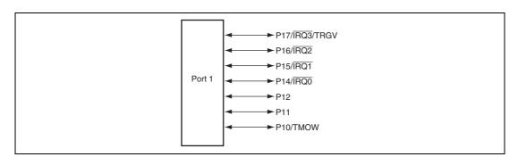
Figure 9.1 Port 1 Pin Configuration
