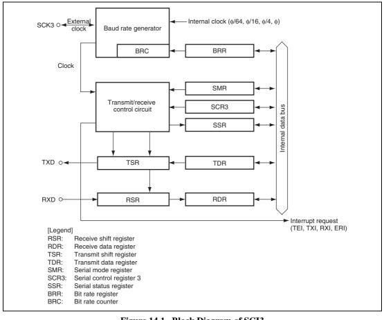
Figure 14.1 Block Diagram of SCI3
