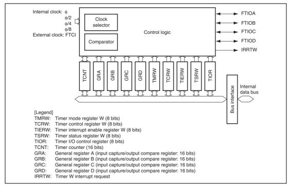
Figure 12.1 Timer W Block Diagram
