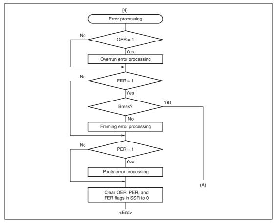
Figure 14.8 Sample Serial Reception Data Flowchart (2)
