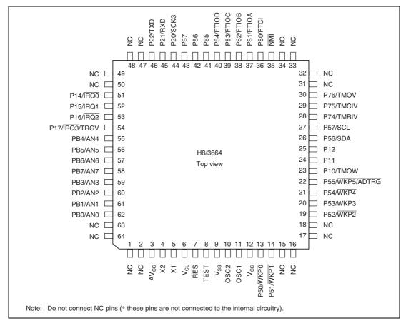
Figure 1.3 Pin Arrangement of H8/3664 of F-ZTAT<sup>™</sup> and Mask-ROM Versions (FP-64E, FP-64A)
