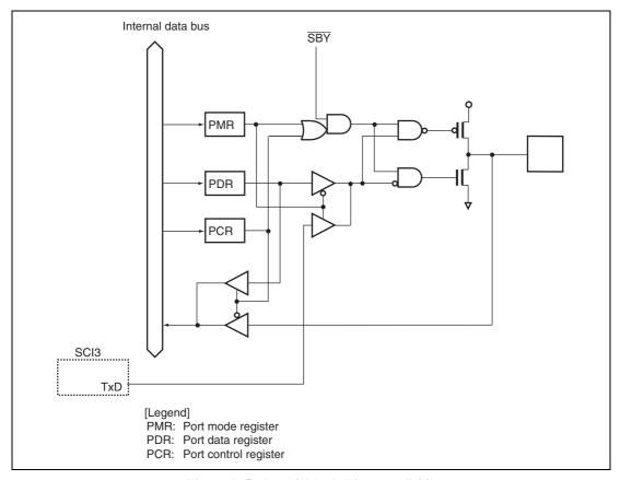
Figure B.5 Port 2 Block Diagram (P22)
