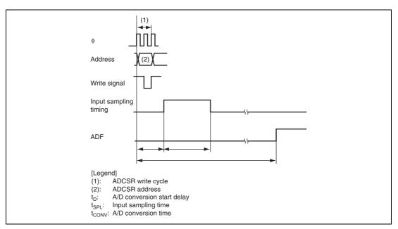
Figure 16.2 A/D Conversion Timing
