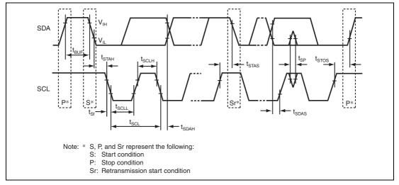
Figure 20.4 I<sup>2</sup>C Bus Interface Input/Output Timing
