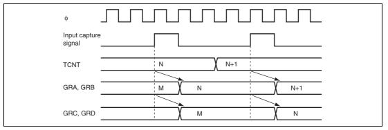
**Figure 12.20 Buffer Operation Timing (Input Capture)**
