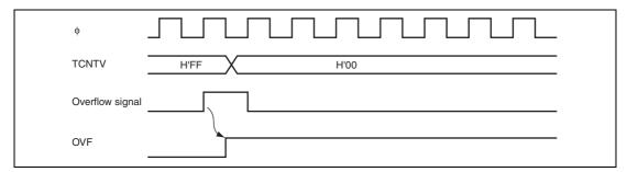
Figure 11.4 OVF Set Timing
