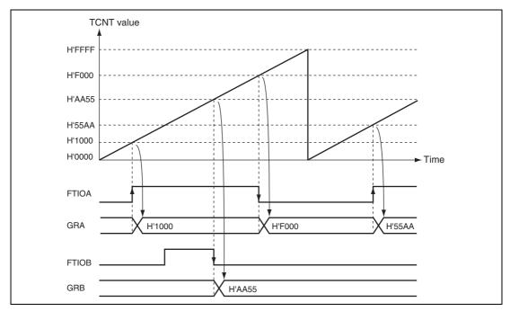
Figure 12.7 Input Capture Operating Example
