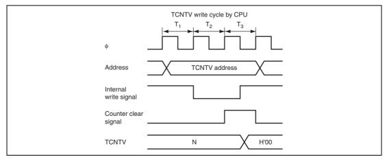
Figure 11.11 Contention between TCNTV Write and Clear
