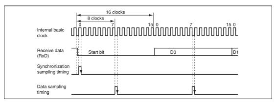
Figure 14.19 Receive Data Sampling Timing in Asynchronous Mode
