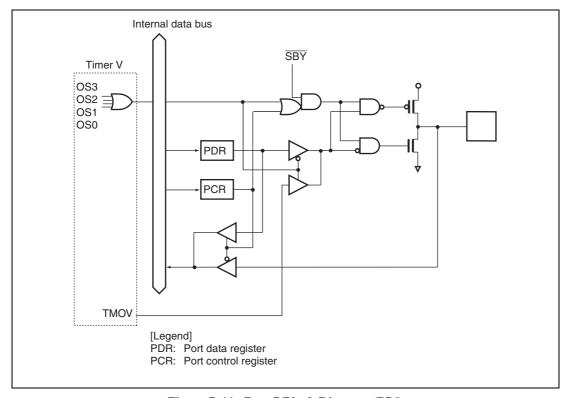
Figure B.11 Port 7 Block Diagram (P76)
