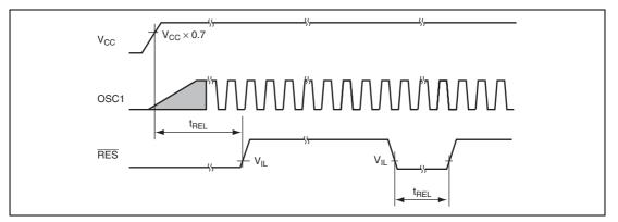
Figure 20.2 RES Low Width Timing
