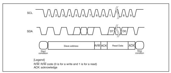
Figure 17.5 Current Address Read Operation
