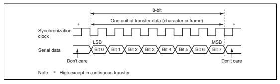
Figure 14.9 Data Format in Clocked Synchronous Communication
