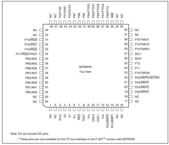
Figure 1.6 Pin Arrangement of H8/3664N of F-ZTAT<sup>™</sup> Version with EEPROM (FP-64E)
