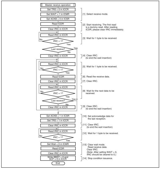
Figure 15.14 Sample Flowchart for Master Receive Mode
