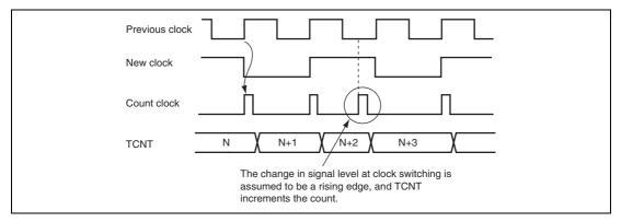
Figure 12.25 Internal Clock Switching and TCNT Operation
