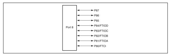
Figure 9.5 Port 8 Pin Configuration
