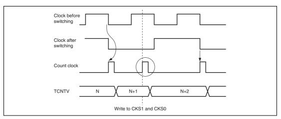
Figure 11.13 Internal Clock Switching and TCNTV Operation
