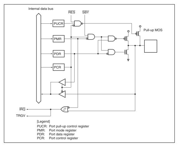
Figure B.1 Port 1 Block Diagram (P17)
