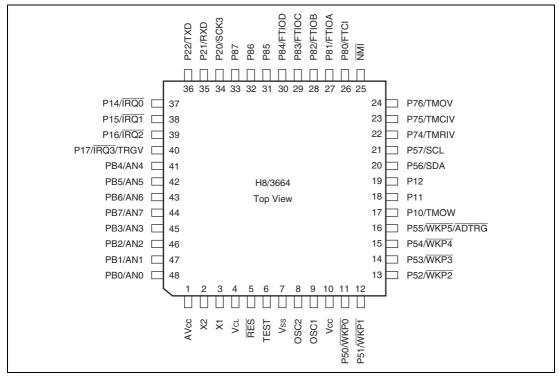
Figure 1.4 Pin Arrangement of H8/3664 of F-ZTAT $^{\text{TM}}$  and Mask-ROM Versions (FP-48F, FP-48B)
