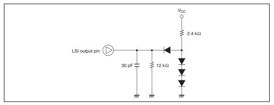
Figure 20.8 Output Load Circuit
