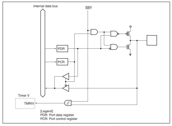
Figure B.13 Port 7 Block Diagram (P74)
