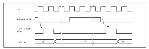
Figure 11.2 Increment Timing with Internal Clock
