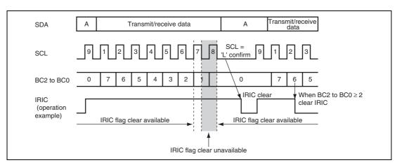
Figure 15.18 IRIC Flag Clear Timing on WAIT Operation
