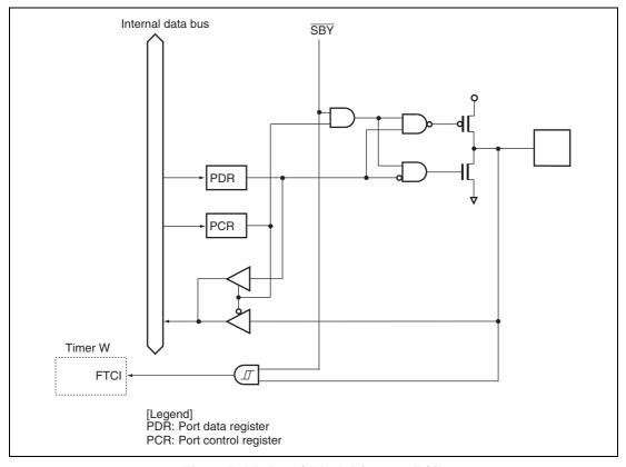
Figure B.16 Port 8 Block Diagram (P80)
