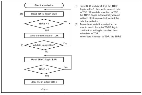
Figure 14.11 Sample Serial Transmission Flowchart (Clocked Synchronous Mode)
