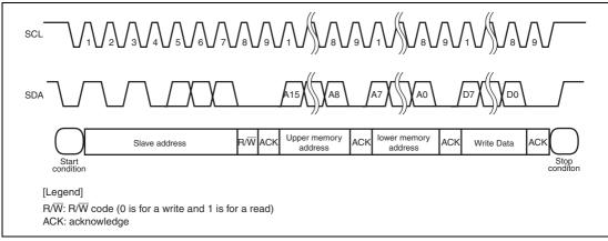
Figure 17.3 Byte Write Operation
