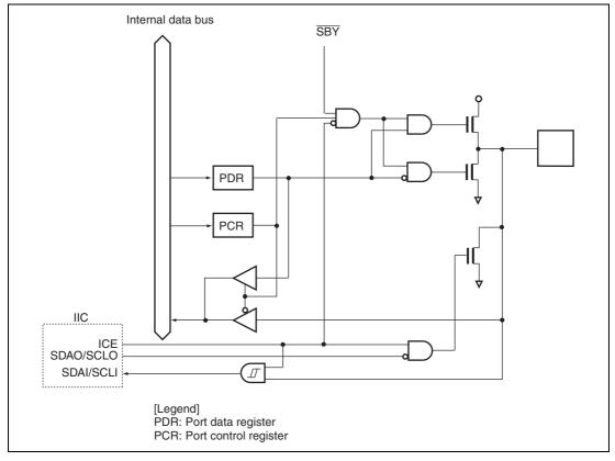
Figure B.8 Port 5 Block Diagram (P57, P56)\*
