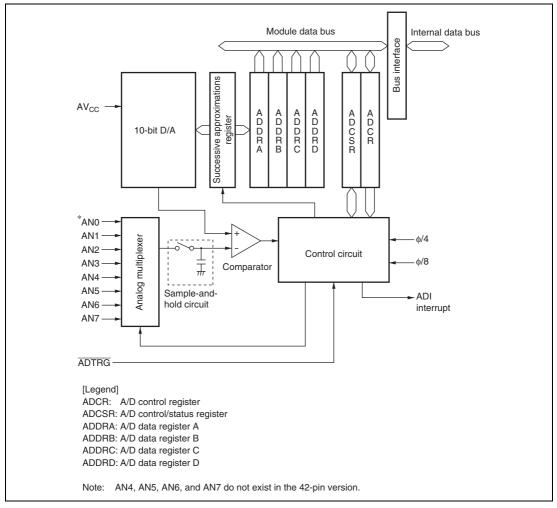
Figure 16.1 Block Diagram of A/D Converter
