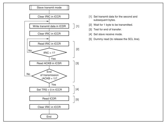
Figure 15.16 Sample Flowchart for Slave Transmit Mode
