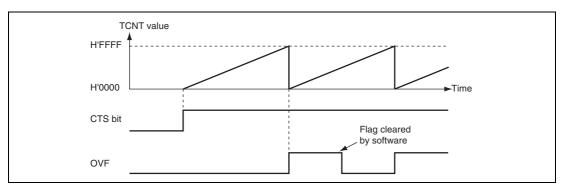
Figure 12.2 Free-Running Counter Operation
