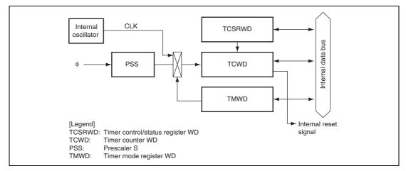
Figure 13.1 Block Diagram of Watchdog Timer
