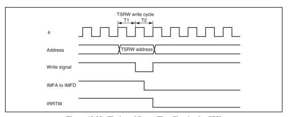
Figure 12.23 Timing of Status Flag Clearing by CPU
