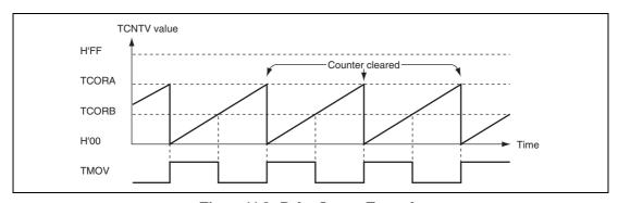
Figure 11.9 Pulse Output Example
