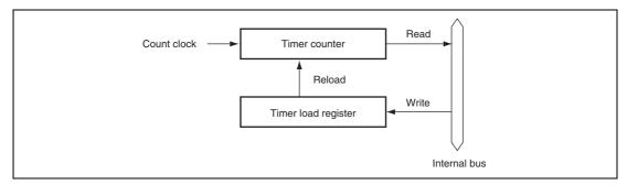
Figure 2.13 Example of Timer Configuration with Two Registers Allocated to Same Address
