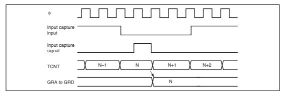
Figure 12.17 Input Capture Input Signal Timing
