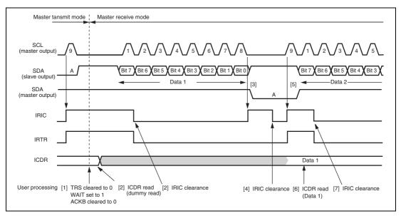
Figure 15.6 Master Receive Mode Operation Timing Example (1) (MLS = ACKB = 0, WAIT = 1)
