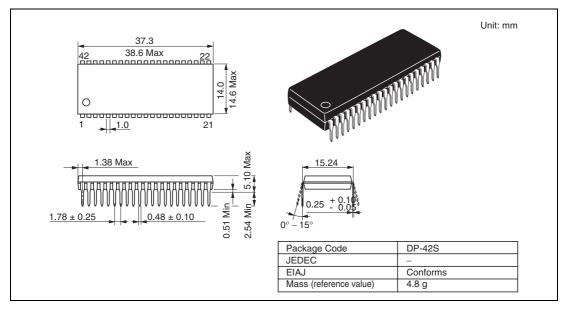
Figure D.5 DP-42S Package Dimensions
