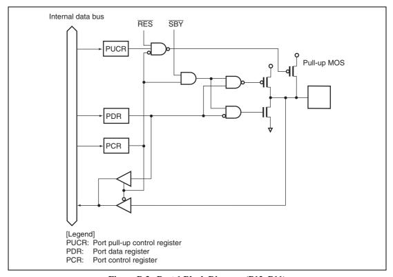
Figure B.3 Port 1 Block Diagram (P12, P11)
