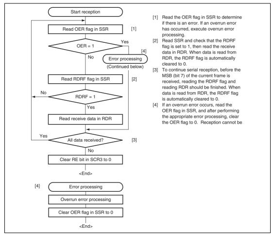
Figure 14.13 Sample Serial Reception Flowchart (Clocked Synchronous Mode)
