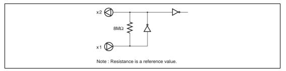
Figure 5.7 Block Diagram of Subclock Generator
