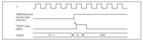
Figure 11.8 Clear Timing by TMRIV Input
