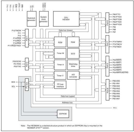
Figure 1.2 Internal Block Diagram of H8/3664N of F-ZTAT<sup>™</sup> Version with EEPROM
