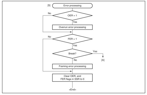
Figure 14.17 Sample Multiprocessor Serial Reception Flowchart (2)
