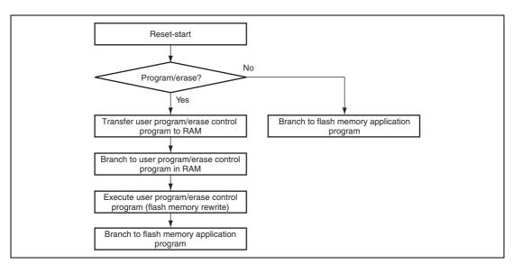
Figure 7.2 Programming/Erasing Flowchart Example in User Program Mode
