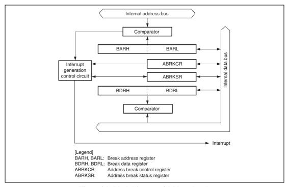
Figure 4.1 Block Diagram of Address Break
