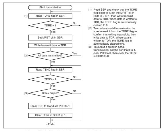
Figure 14.16 Sample Multiprocessor Serial Transmission Flowchart
