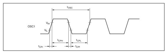
Figure 20.1 System Clock Input Timing
