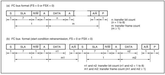
Figure 15.3 I<sup>2</sup>C Bus Data Formats (I<sup>2</sup>C Bus Formats)
