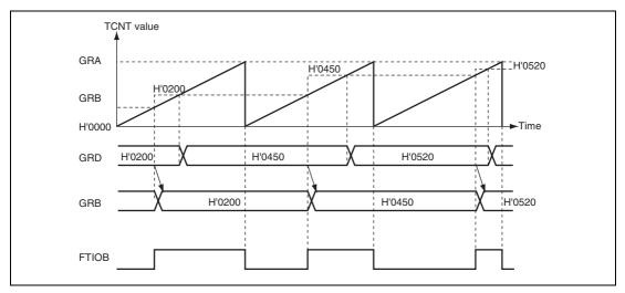
**Figure 12.11 Buffer Operation Example (Output Compare)**
