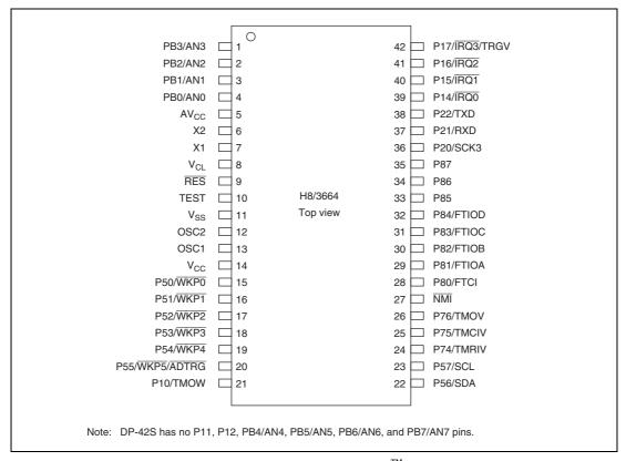
Figure 1.5 Pin Arrangement of H8/3664 of F-ZTAT $^{\text{TM}}$  and Mask-ROM Versions (DS-42S)
