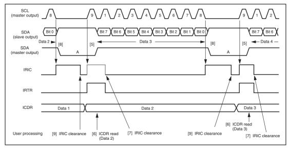
Figure 15.6 Master Receive Mode Operation Timing Example (2) (MLS = ACKB = 0, WAIT = 1)
