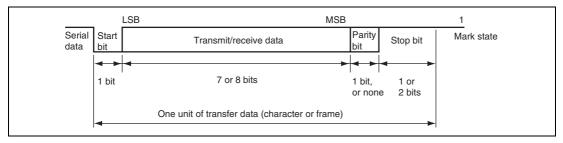
Figure 14.2 Data Format in Asynchronous Communication
