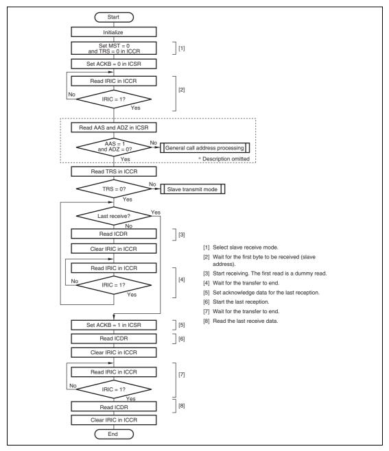
Figure 15.15 Sample Flowchart for Slave Receive Mode
