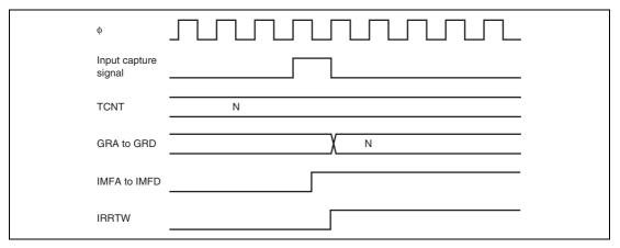
Figure 12.22 Timing of IMFA to IMFD Flag Setting at Input Capture
