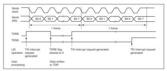
Figure 14.10 Example of SCI3 Operation in Transmission in Clocked Synchronous Mode
