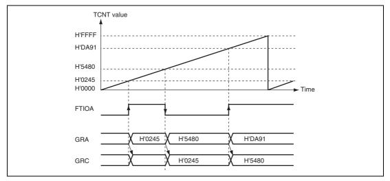
Figure 12.8 Buffer Operation Example (Input Capture)
