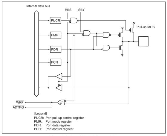
Figure B.9 Port 5 Block Diagram (P55)
