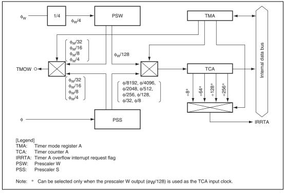
Figure 10.1 Block Diagram of Timer A
