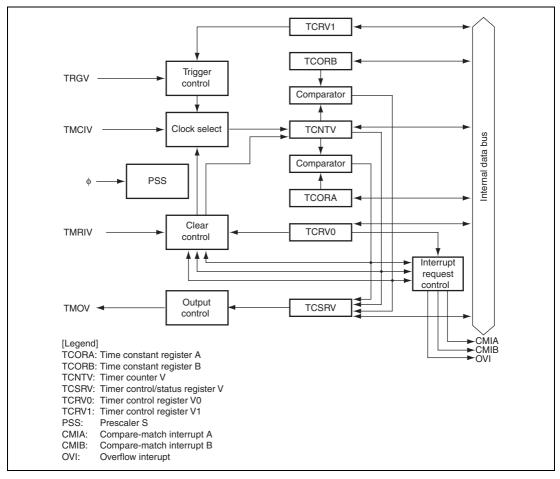
Figure 11.1 Block Diagram of Timer V
