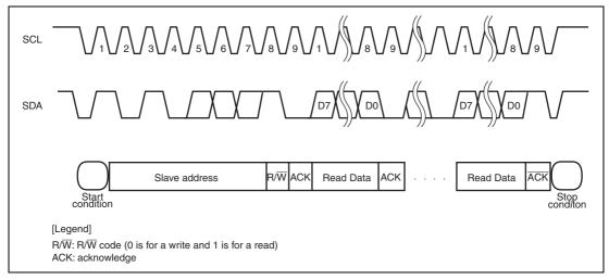
Figure 17.7 Sequential Read Operation (when current address read is used)
