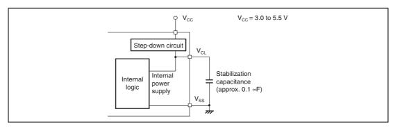
Figure 18.1 Power Supply Connection when Internal Step-Down Circuit is Used
