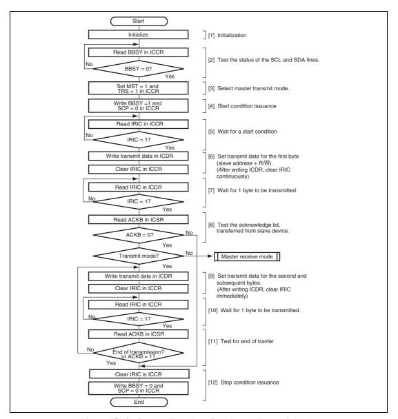
Figure 15.13 Sample Flowchart for Master Transmit Mode
