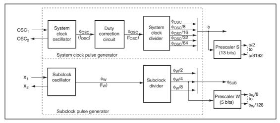
Figure 5.1 Block Diagram of Clock Pulse Generators
