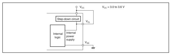
Figure 18.2 Power Supply Connection when Internal Step-Down Circuit is Not Used
