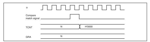
Figure 12.18 Timing of Counter Clearing by Compare Match
