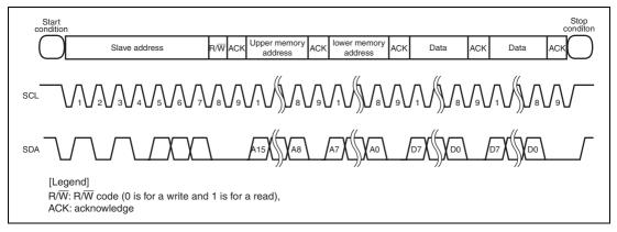
Figure 17.2 EEPROM Bus Format and Bus Timing
