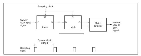
Figure 15.12 Block Diagram of Noise Canceler
