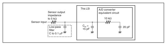
Figure 16.6 Analog Input Circuit Example
