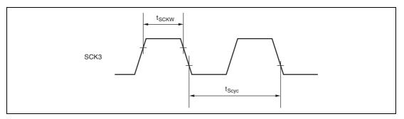
Figure 20.5 SCK3 Input Clock Timing
