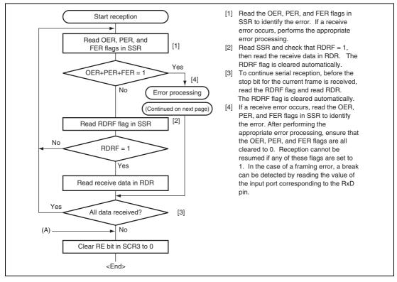
Figure 14.8 Sample Serial Data Reception Flowchart (Asynchronous mode) (1)
