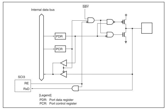
Figure B.6 Port 2 Block Diagram (P21)
