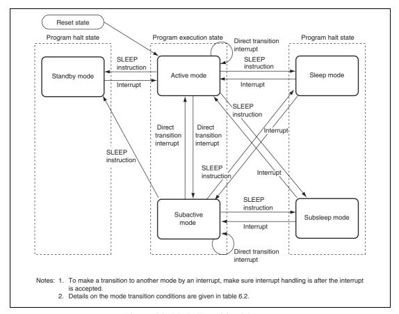
Figure 6.1 Mode Transition Diagram
