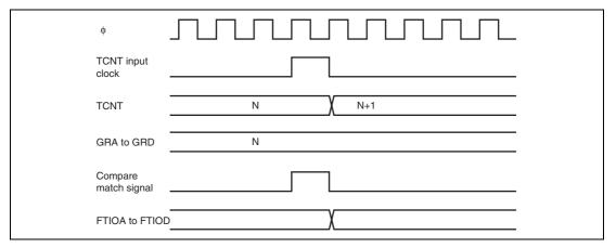
Figure 12.16 Output Compare Output Timing
