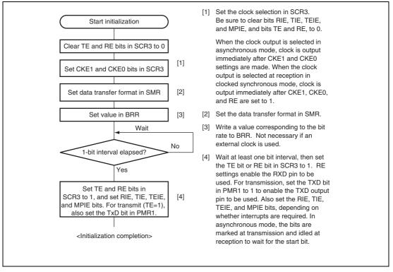
Figure 14.4 Sample SCI3 Initialization Flowchart
