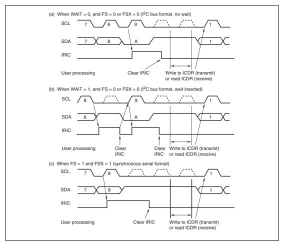
Figure 15.11 IRIC Setting Timing and SCL Control
