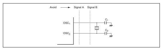
Figure 5.11 Example of Incorrect Board Design
