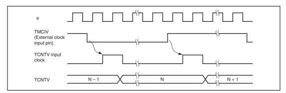
Figure 11.3 Increment Timing with External Clock
